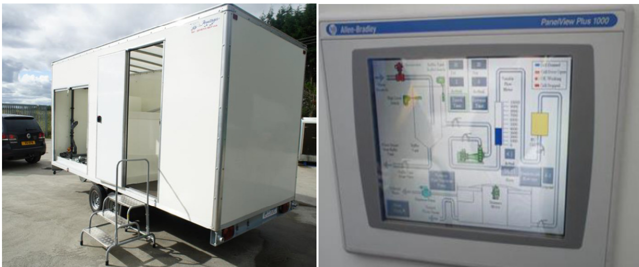
Figure 1: Containerised EC system for use in the UK Oil & Gas Sector
