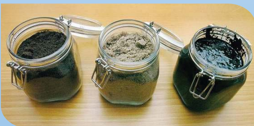
Sand before treatment (Left) Sand after treatment (Centre) Oil recovered (Right)
